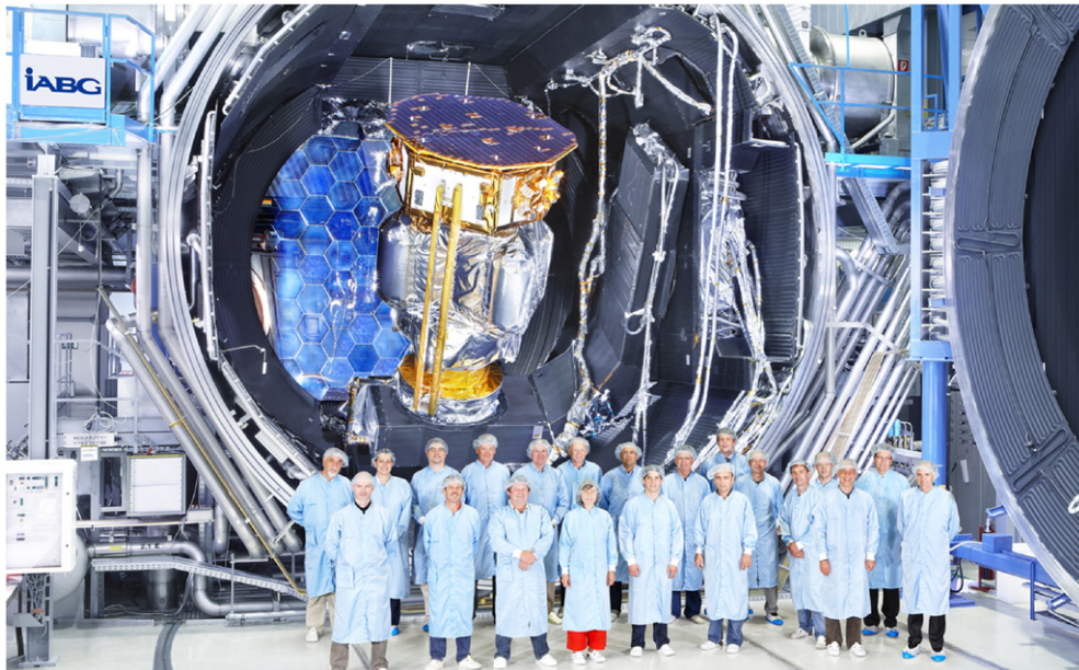
Figure 5. The LISA Pathfinder launch composite being in the vacuum chamber in preparation for the transfer orbit thermal balance test. The test was performed at the IABG, Germany.
