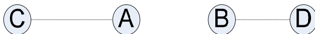
Fig. 1. S-MAC: Neighboring nodes A and B have different schedules. They synchronize with nodes C and D respectively
