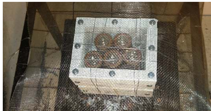
Figure 5. Lifetech single cells before the fire test at 100% SOC with external propane burner.
