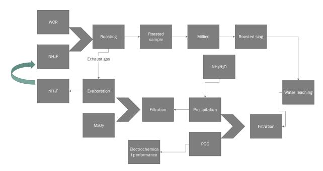
**Figure 10.** Flow diagram of high-purity graphite carbon and metal recovery from WCR, redrawn from Zhu, Xiao, Mao, Zhang, You, Tang and Zhong [106].
