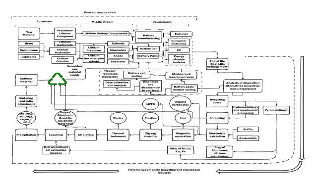
Figure 2. General flow diagram of the recycling process of LIBs, compiled and redrawn from [17–20].
