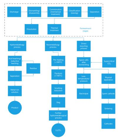
**Figure 7.** Pre-treatment and various recycling processes of waste LIBs (partially adopted from Kim, et al. [104] and Zhou, et al. [105]).
