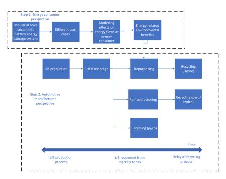
**Figure 12.** Two-step process of battery second-life application for energy storage system and associated business models [44].
