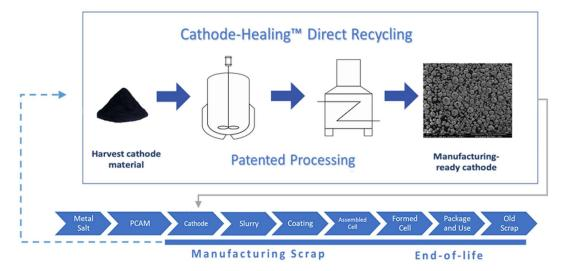
Figure 11. Cathode-Healing Direct recycling technology for spent LIBs by OnTo Technology (USA), adapted from [107].
