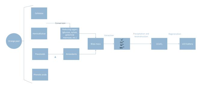
**Figure 8.** Mechanism and process summary of recycling of spent LIBs using orange peel (), redrawn from Wu, Soh, Chan, Meng, Meyer, Srinivasan and Tay [62].
