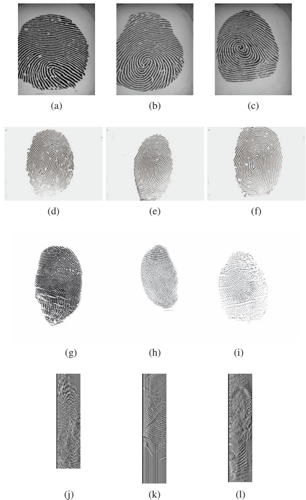
Figure 1: Examples of acquired fake fingerprints. Non-cooperative: Biometrika (a, b, c); Italdata (d, e, f). Cooperative: Crossmatch (g, h, i); Swipe (j, k, l). Cast materials: gelatine (a, d); latex (b, e, h, k); wood glue (c, f, i, l); body double (g, j).
