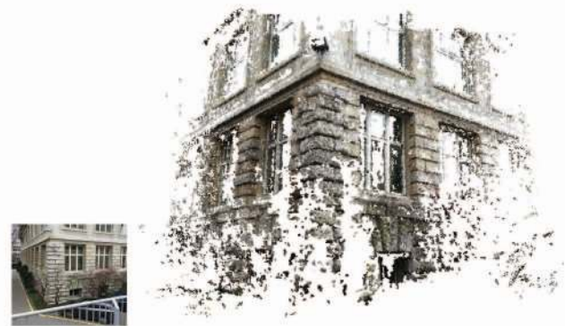
Figure 8. Photo and reconstructed 3D model of a building facade captured at street-level.
