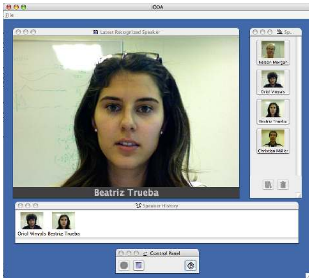
Figure 2: Screenshot of the Java GUI that embeds the online speaker identification system. The system shows the face and the name of the current speaker, along with the time line (bottom) and the pool of trained speakers (right).
