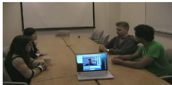
Figure 1: The demonstrated system at work: A laptop is recording the meeting and identifying speakers as they talk. Only the laptop's internal microphone is used and the system works text- and language independent.
