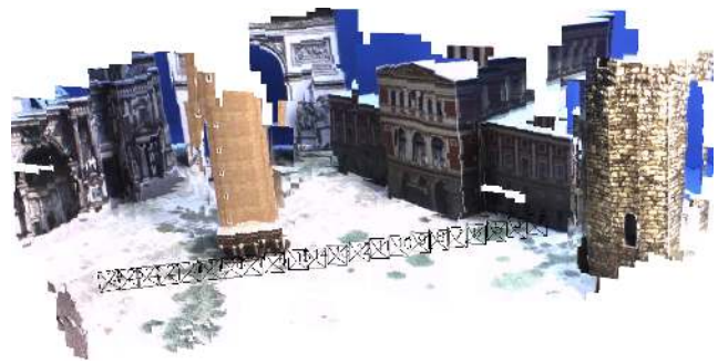
Figure 9: Our system acting as a SLAM system, reconstructing the scene in 3D and recovering the camera trajectory fully automatically. The input sequence for this model stems from the “City of Sights” repository [12] and was recorded by a robot arm. Each reconstructed 3D feature position is visualized as a small image patch (sampled from the frame in which it was first observed).
