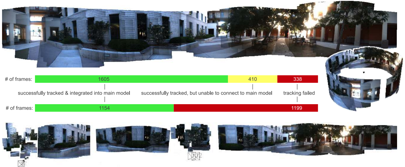
Figure 5: Merging of tracks (top) vs. relocalization (bottom). The rotation-only input video for the data shown here contains several rapid camera motions (cf. description of the dataset in [6]), resulting in intermittent tracking loss. After each loss, our system starts a new partial panorama, and, while the incoming live frames are being processed, attempts to stitch them together in the background. The final panorama (top) is an almost complete horizontal panorama of the scene (cf. cylindrical rendering on the right). 1605 frames are registered to this panorama. Another 410 frames are registered to partial panoramas (not shown) which the system was unable to connect to the main model (whether these should be counted as success or failure depends on the application that the system is used for). For 338 frames, tracking failed. In comparison, with the same tracking system but using relocalization, only the model at the bottom gets mapped, with 1154 registered frames. (Here, the model is visualized in five segments because the transition between two pairs of keyframes got modeled with an essential matrix, but the model is—by construction—fully connected.) The data of all other 1199 frames (which “passed by” while the system unsuccessfully tried to relocalize) are discarded.
