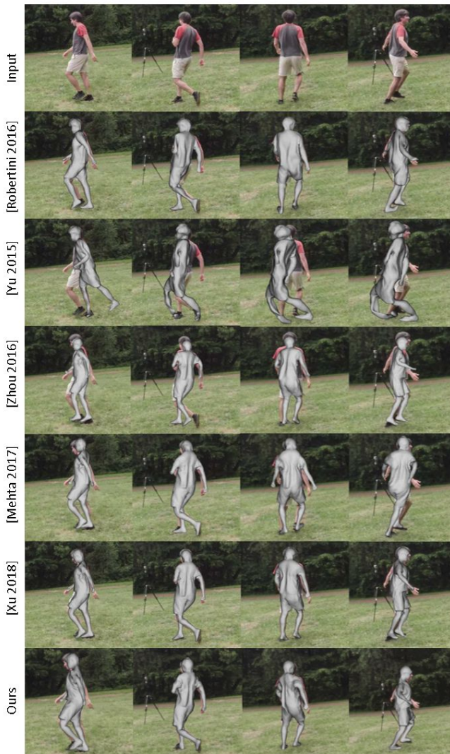
Fig. 12. Qualitative comparisons of the surface reconstruction accuracy on the Pablo sequence. Our real-time monocular approach comes very close in quality to the results of the fundamentally off-line multi-view approach of Robertini et al. [2016] and the monocular off-line method of Xu et al. [2018]. It clearly outperforms the monocular non-rigid capture method of Yu et al. [2015] and the rigged skeleton-only results of the 3D pose estimation methods of Zhou et al. [2016] and Mehta et al. [2017].
