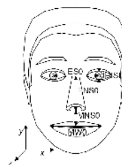
Figure 1. A face model in its neutral state and defined FAP units (FAPU) (ISO/IEC IS 14496-2 Visual, 1999)
