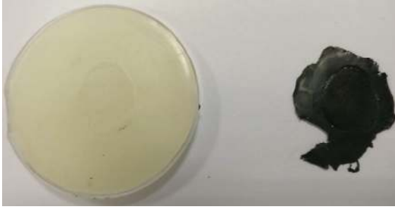
Figure 4: Artificial fingerprint replica. The left is the mold used to capture fingerprint; the right is a fake fingerprint crafted using silicone rubber.
