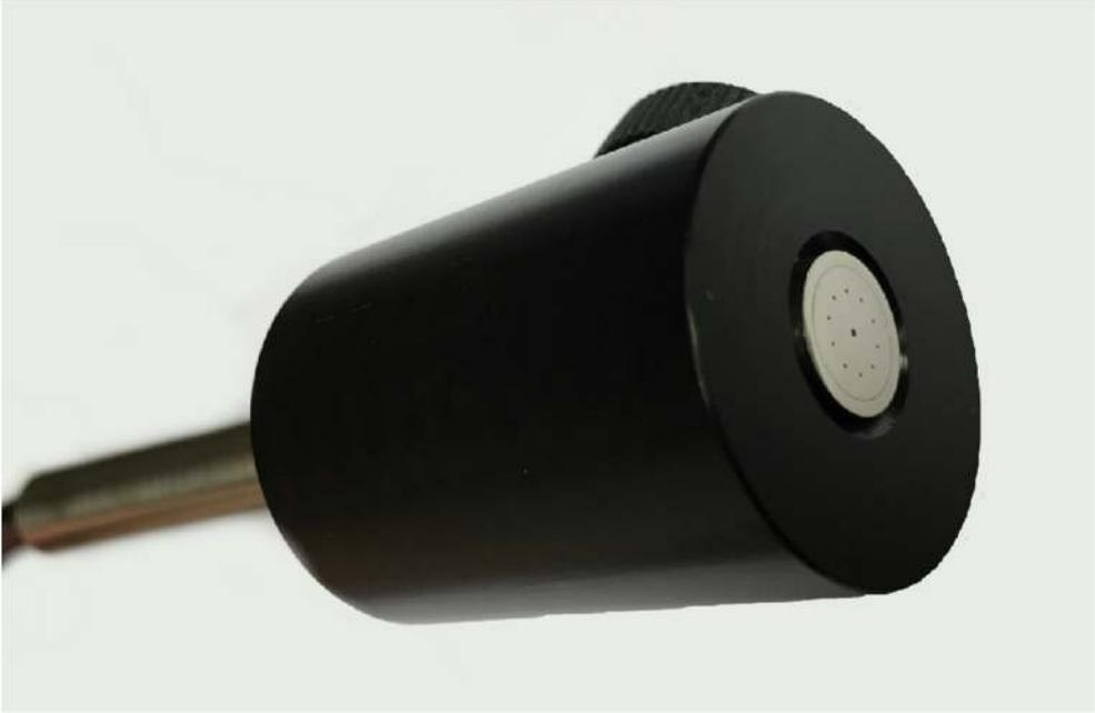
**Figure 13.** Picture of the hand-held probe including the 25 mm diameter probe cylinder (black part) attached at the top.
