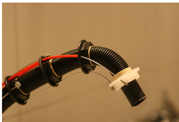
Figure 1. Prototype, tube bent by steel wires
