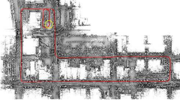
Figure 4. Trajectory (in red) and the built map of LO-Net+Mapping on Ford dataset 1. Our reconstructed trajectory (without enforcing loop closure) has small drift and forms closed loops accurately (yellow circle).
