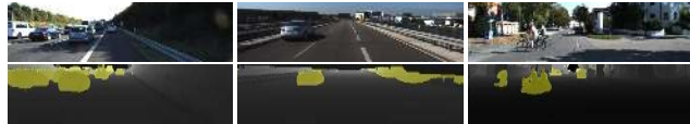
Figure 9. Sample visualizations of masks on range channel of the data matrix and its corresponding RGB images. The yellow pixels indicate the uncertain points in the surrounding environment for odometry estimation, such as points of moving cars, cyclists and others. The images are cropped and reshaped for better visualization.
