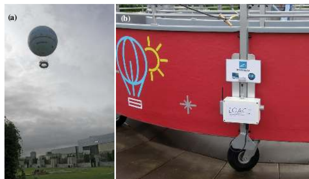
Figure 7. LOAC on the recreational OAG tethered balloon in Parc André Citroën, Paris. (a) View on the balloon in flight; (b) view of the LOAC installed in a small box on the side of the passenger gondola with its TSP inlet above, a small WiFi antenna on the left of the box for data transmission, and a ventilation opening protection (grey) on the right.
