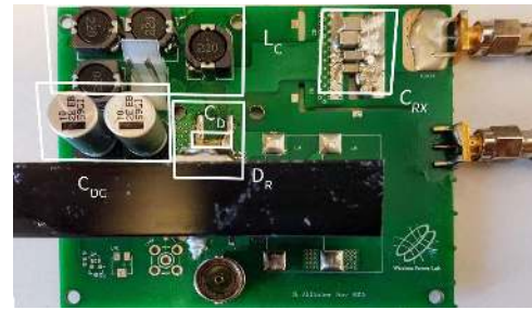
Fig. 12. Photograph of the Class-E rectifier.
