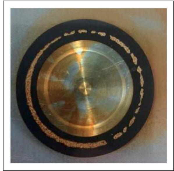
Figure 17. This figure presents the ferrofluid pocket bearing used for the experiment discussed in this section. With a glass plate, the two seals with capillary interconnection are made visible. The magnet used is the HKCM 9963-433.
