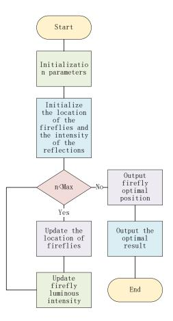
Figure 2. The flow chart of the firefly algorithm.
