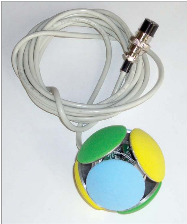
Fig. 4. Sphere shaped load cell.
