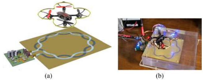
Fig. 31. Setup and implementation of the wirelessly powered drone. (a) Setup. (b) Demonstration.
