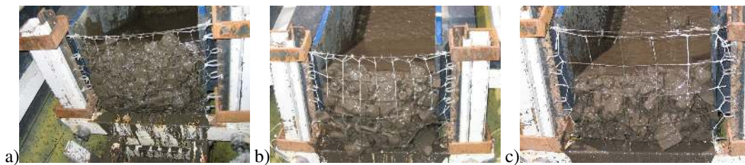
Fig. 3. Small-scale net barriers with different mesh sizes after laboratory tests (Wendeler and Volkwein, 2015): (a) 3 cm mesh size kept nearly the same amount of material as (b) 4 cm mesh size. (c) The retained volume with the 6 cm mesh size is only two thirds compared to the two other mesh sizes.
