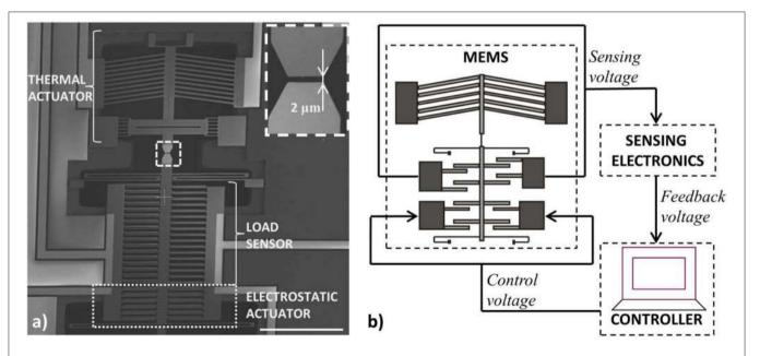
FIGURE 2 | (a) SEM picture of the tensile testing device proposed in Pantano et al. (2015) provided with load sensor feedback control. It consists of a thermal actuator, a capacitive load sensor, and an electrostatic actuator. The thermal actuator and the load sensor are separated by a 2 μm gap for accommodation of the sample to be tested (zoomed view on top); (b) Implementation of the feedback voltage control scheme for keeping the load sensor at rest during test on a sample. Scale bar: 500 μm.
