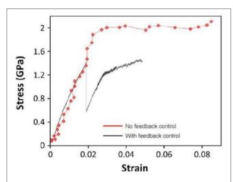
**FIGURE 3** | Stress-strain curves derived from tensile tests on silver nanowires of 118 nm diameter. The red curve is referred to a test where the load sensor is allowed to move, while the black curve was derived during a test where a displacement feedback control of the load sensor was implemented. Reprinted with permission from Pantano et al. (2015). Copyright 2015, Springer.
