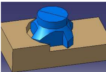
Fig. 7. Three dimensional graphics of a face milling cutter
