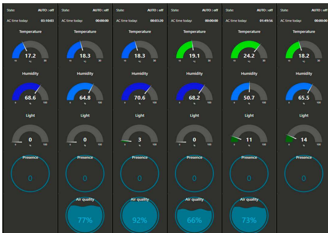
Figure 8. Node-RED Dashboard, indicators and real time consumption view.
