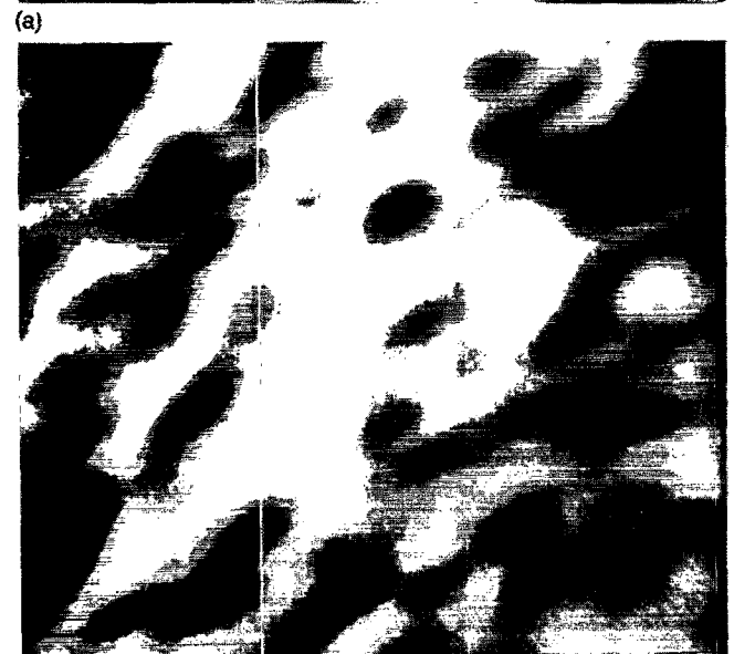
FIG. 4. (a) NIR (wavelength above 1000 nm) and (b) visible CL images of the same area of an as-grown sample. Arrows indicate two emergence points of dislocations.
