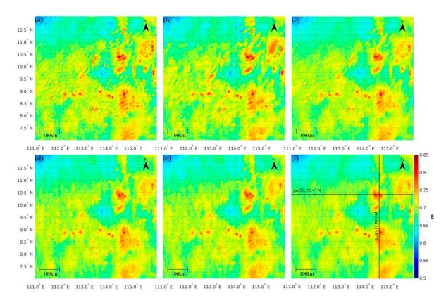
**Figure 6.** MDTs derived from the quasi-geoid model computed from (**a**) XGM2019e\_2159, (**b**) HY2A, (**c**) SCSGA, (**d**) SIO30, (**e**) SIO31, and (**f**) DTU21GRA. The geographical coordinates are expressed in the Plate Carrée projection. Note: only SIO30, SIO31, and DTU21GRA were computed with the SAR altimetry data derived from Sentinel-3A/B over the study area.
