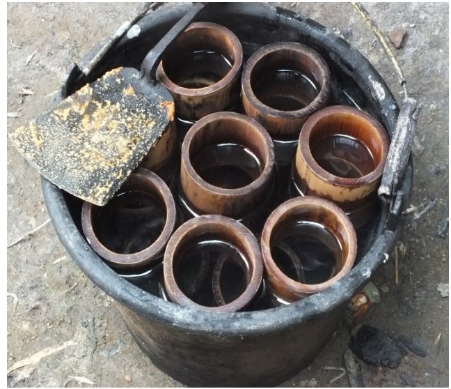
Figure 8. The liquid is poured into bamboo internodes to be molded
