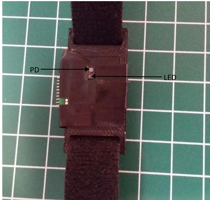
Figure 2.3 The PPG sensor armband with the vinyl cover. The arrows indicate the PD and LED.
