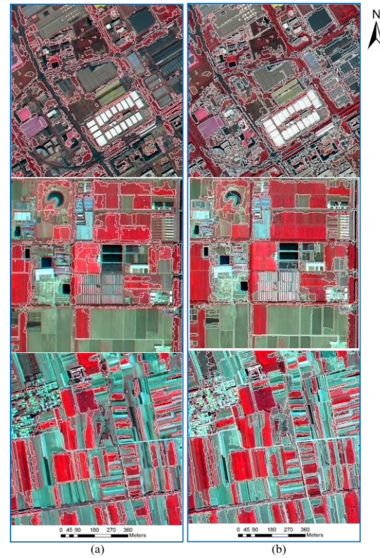
FIGURE 10. The local scale-guided region merging results of the test images at the optimal \beta : (a) vegetative merging results, and (b) non-vegetative merging results.
