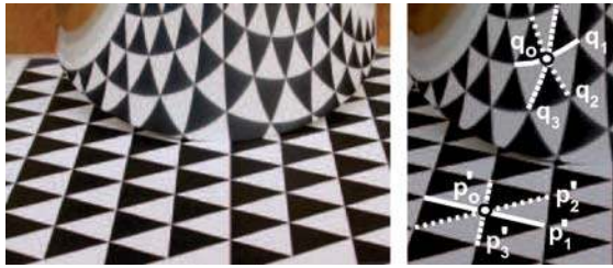
Figure 6. Data gathered from the image. In this example the measurements are the orientations of the reflected curves \mathbf{q}_1 , \mathbf{q}_2 and \mathbf{q}_3 evaluated at the intersecting point \mathbf{q}_0 and the position of \mathbf{q}_0 in the image plane.
