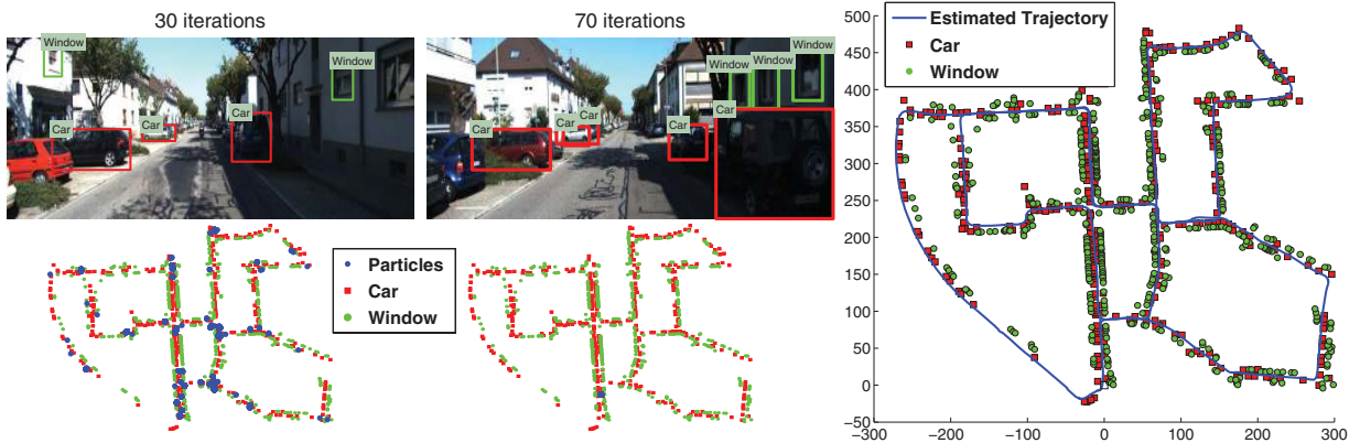
Fig. 18. Vehicle trajectory estimated via global semantic localization on sequence 00 from the KITTI visual odometry dataset. The left and middle plots show two images with car and window detections and the corresponding particle distributions in the semantic map. The plot on the right shows the semantic map and the trajectory, recovered after unique localization (iteration 70). See Extensions 5 and 6 for more details.
