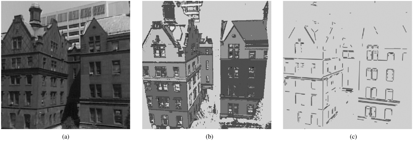
Fig. 19. Model acquisition and simplification. (a) An image of a building. (b) The 3-D model created from the image and a range scan. (c) A reduced version of the same model consisting only of line features.
