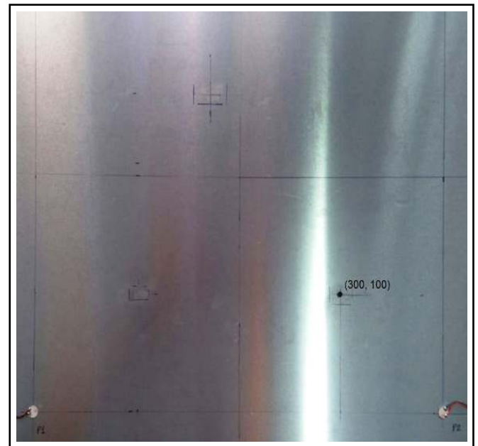
Figure 29. A through thickness hole in the plate.
