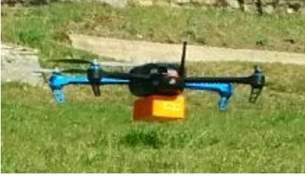
Fig. 1. UAV and RFID reader.
