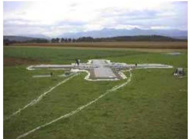
Fig. 2 Array of microphones. Flight-path is from left foreground to right background.
