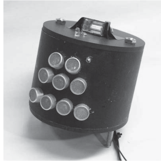
Figure 3: The “Pinger” delivers a simultaneous flash of light and burst of 40-kHz ultrasound. Each Pushpin can measure the difference in time of arrival of these two signals and thus calculate the distance between itself and the Pinger.
