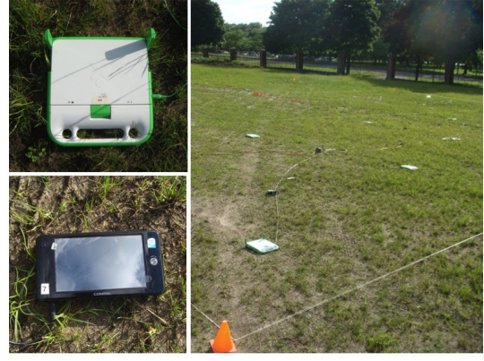
Figure 9: Photo of outdoor testbed with 21 OLPCs (upper left) and 16 MIDs (lower left). These nodes are configured in a “C” topology, on a 25\text{m} \times 25\text{m} open field (right).
