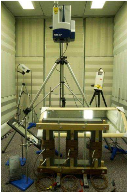
Fig. 3. Transformer core and vibrometer set up in the hemi-anechoic chamber.
