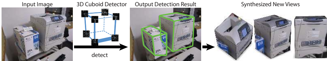
Figure 1: Problem summary. Given a single-view input image, our goal is to detect the 2D corner locations of the cuboids depicted in the image. With the output part locations we can subsequently recover information about the camera and 3D shape via camera resectioning.
