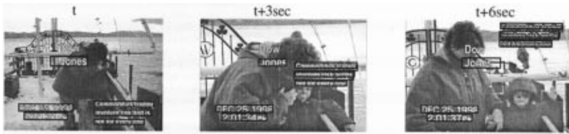
Fig. 9. Example of text tracking of located text lines. All text lines except “Dow” could be successfully tracked. The line “Dow” is missed due to its difficult background (iron gate and face border).
