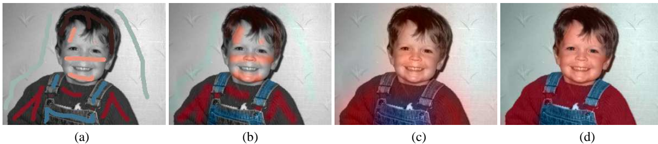
Figure 1: Piecewise smooth color interpolation in a colorization application: (a) input gray image with color strokes overlaid; (b) solution after 20 iterations of conjugate gradient; (c) using 1 iteration of hierarchical basis function preconditioning; (d) using 1 iteration of locally adapted hierarchical basis functions.
