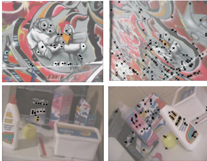
Fig. 4. Image pairs and detected points used in homography experiments (D and E). Inliers are marked as dots in left images and outliers as crosses in right images.
