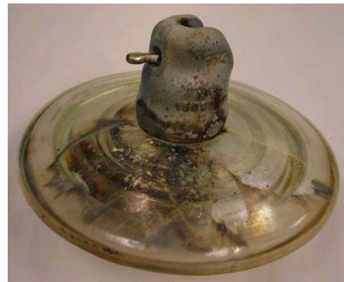
Fig. 29. Damaged insulator at 61.41 km from the Goshen terminal.
