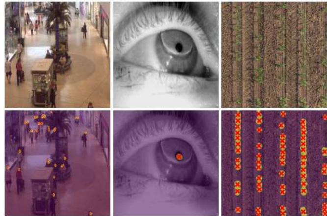
Figure 1. Object localization with human heads, eye pupils and plant centers. (Bottom) Heat map and estimations as crosses.
