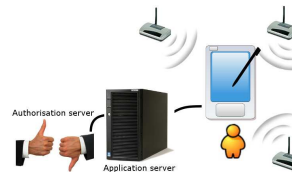
(c) The device determines whether it is within specified range of a set of APs specified in the license
