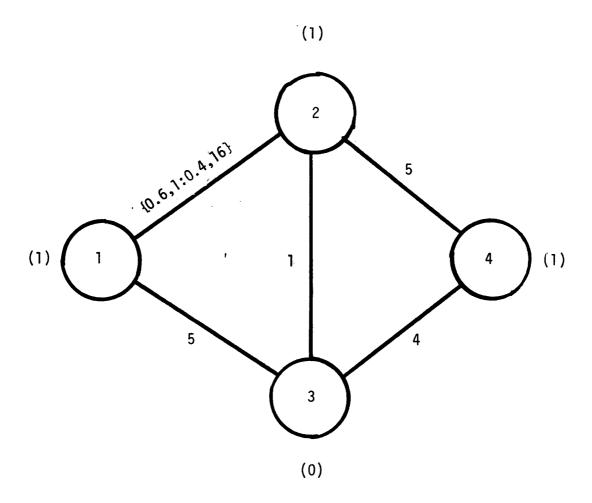
Example of a stochastic network. Link (1,2) has 0.6 probability of 1 unit in travel time and 0.4 probability of 16 units in travel time. The rest of the links have constant travel times. Nodes 1, 2, and 4 have demand weights of 1 unit each and node 3 of 0 units as indicated by the numbers in parentheses.
