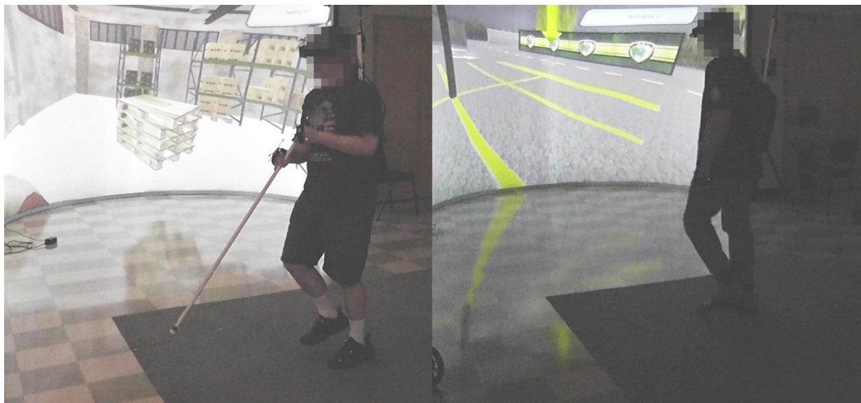
Figure 3-4: Pictures of the walk-in-place locomotion technique in the VR4VR system. The user navigates in the virtual environment by walking in place in the actual world. Cleaning module (left), environmental awareness module (right).
