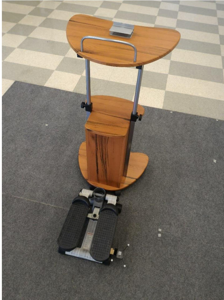
Figure 4-27: The stepper machine, the marker attachment and the holding stage.
