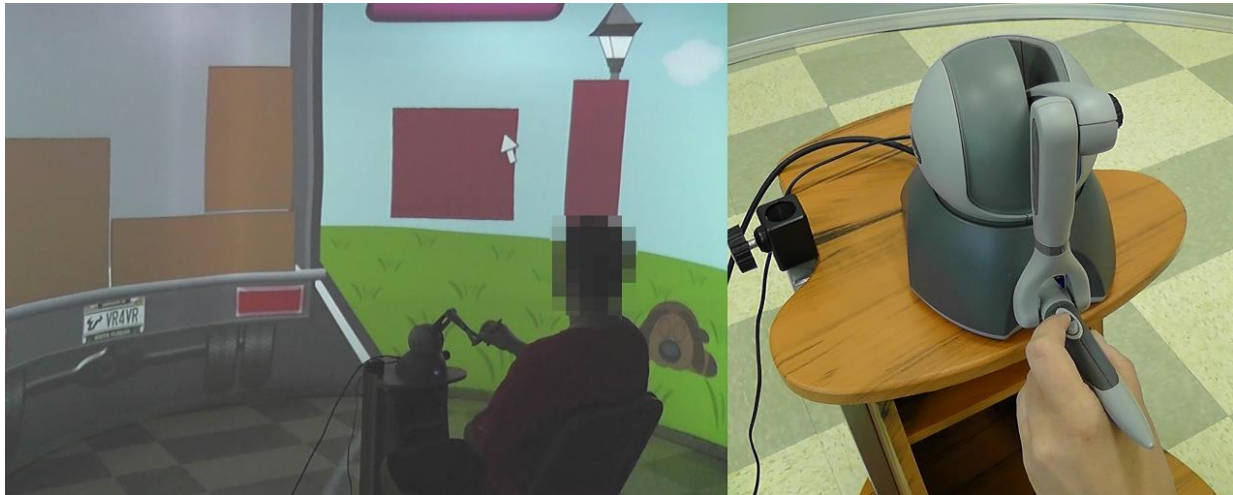
Figure 3-7: The haptic device interaction in the VR4VR system. The user controls the cursor in the virtual world by using the haptic device (left). Haptic device with two buttons on the handle (right).
