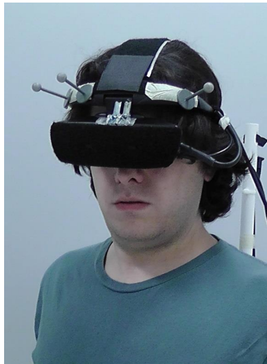
Figure 3-10: Head mounted display in the VR4VR system. The user is wearing the head mounted display with reflective markers on top.
