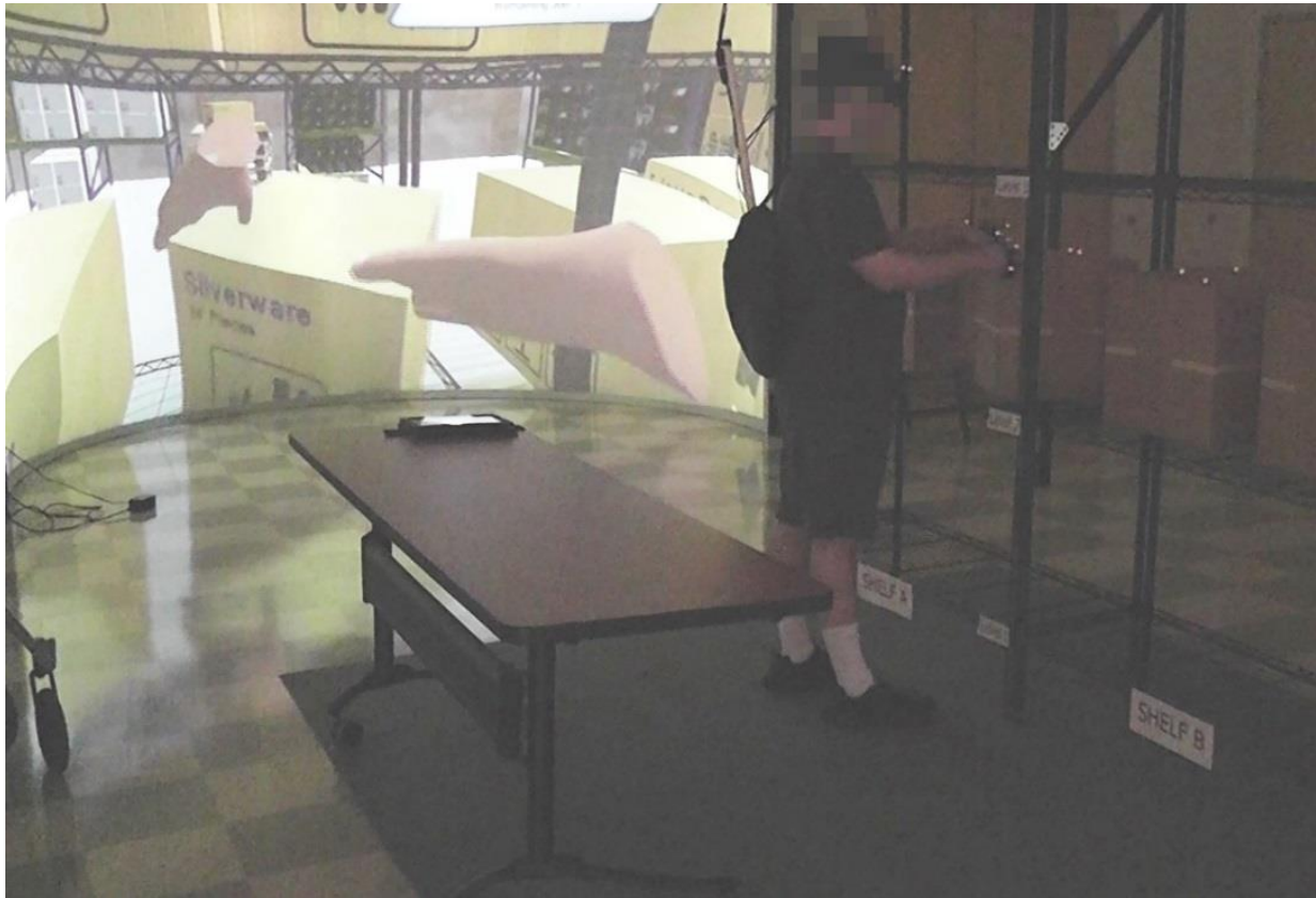
Figure 3-5: Tangible box manipulation in the VR4VR system. The user is rotating a real box. The curtain screen displays the user's view through the HMD.
