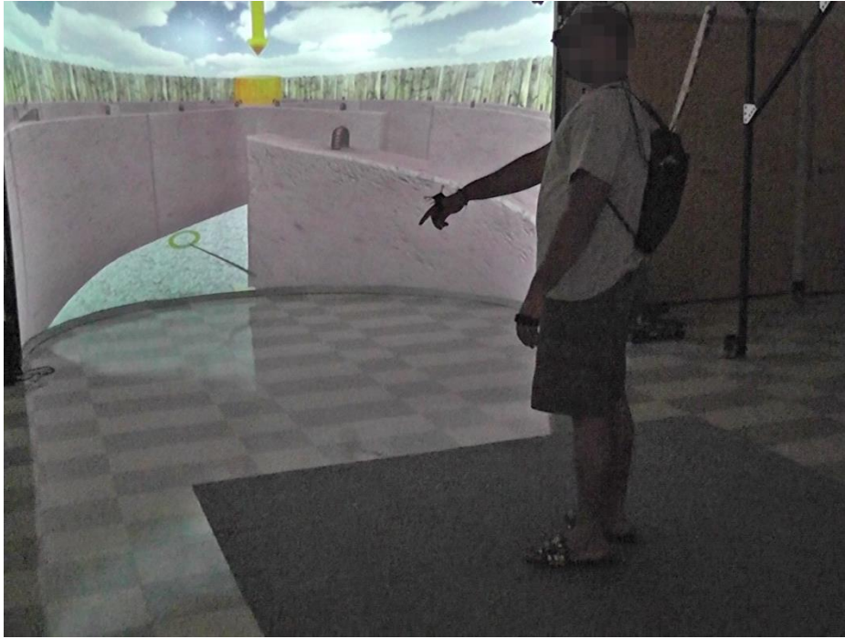
Figure 6-3: Photo of a testing session with the point & teleport locomotion technique in the virtual maze.
