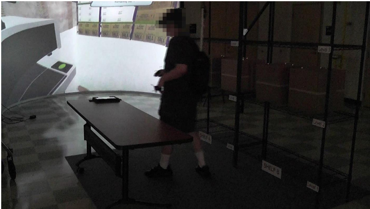
Figure 3-2: Picture of the real walking locomotion technique in the VR4VR system. The user walks inside the tracked area in the shelving module.
