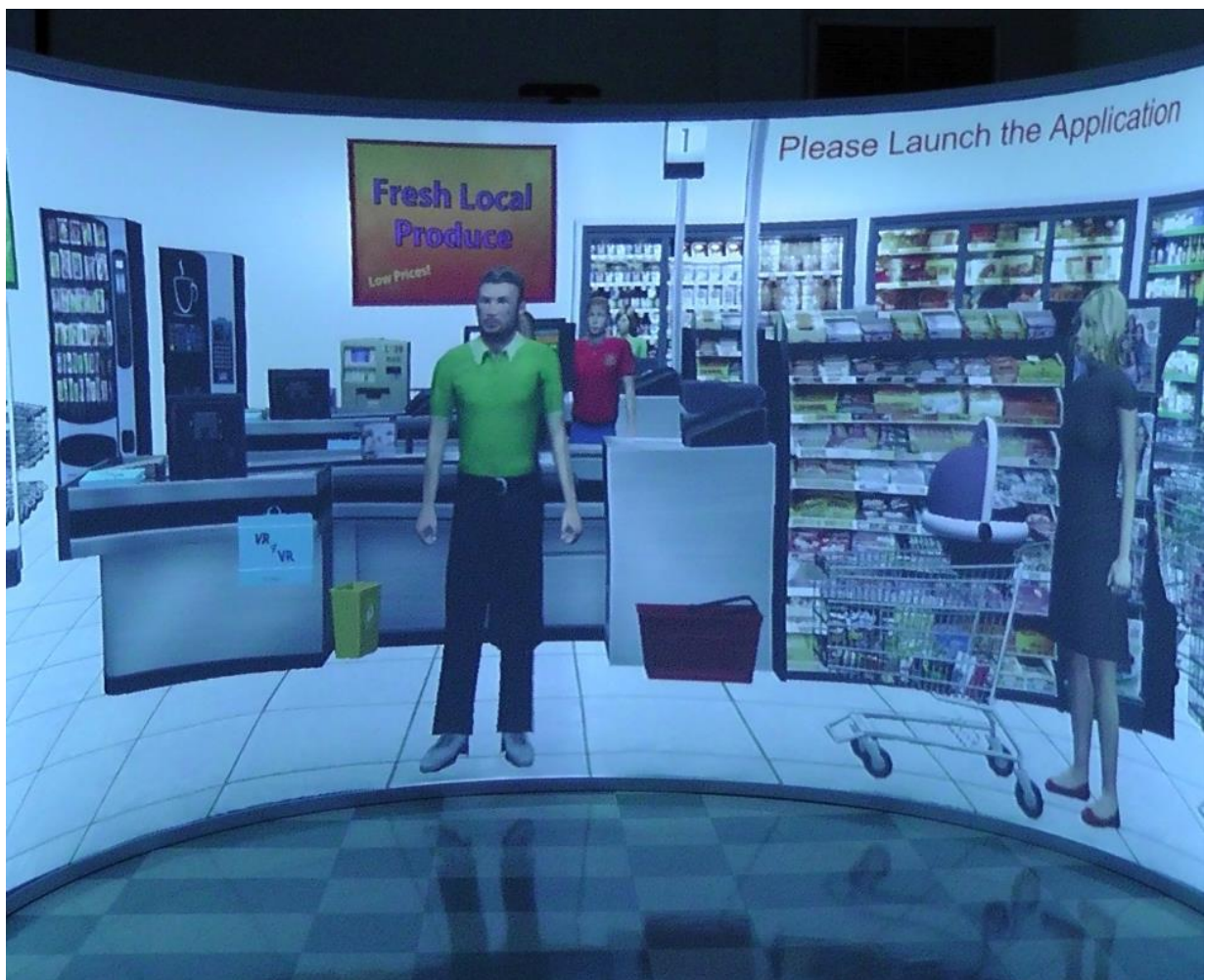
Figure 3-11: Curtain display in the VR4VR system. The virtual grocery store was projected onto the 180 degrees curtain display.
