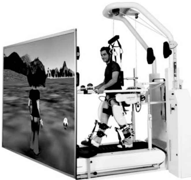
Figure 4. Walking through a virtual environment. Lokomat in combination with a virtual reality system.
