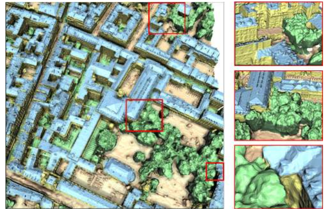
Fig. 8. Classification into four classes of urban elements. The regularizing term of the energy as well as the semantic rules improve spatial consistency. The close-ups depict how roofs and facades, as well as trees adjacent to facades, are adequately separated.
