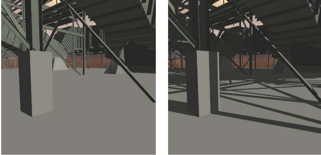
Figure 1.2: Shadows in an interactive walk-through. (Left) Without shadows the structures of this power plant model seem to float above the ground plane. (Right) Shadows aid spatial understanding and add realism.
