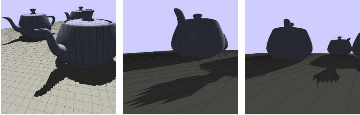
Figure 5.13: Shearing artifacts from a standard shadow map. (Left) With the ground plane oriented nearly perpendicular to the light direction the texel projections visible at shadow edges are rectangular. (Middle) With the ground plane oriented nearly parallel to the light, the texel projections become extremely sheared. These tend to be more disturbing than rectangular texel projections. (Right) From a different point of view, however, the texel projections appear less sheared.
