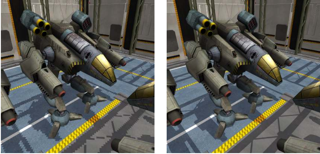
Figure 1.6: Shadow map artifacts. (Left) In this image rendered with a standard shadow map the shadow boundaries are jagged. (Right) The same image rendered with our shadow map algorithm without shadow map artifacts .
